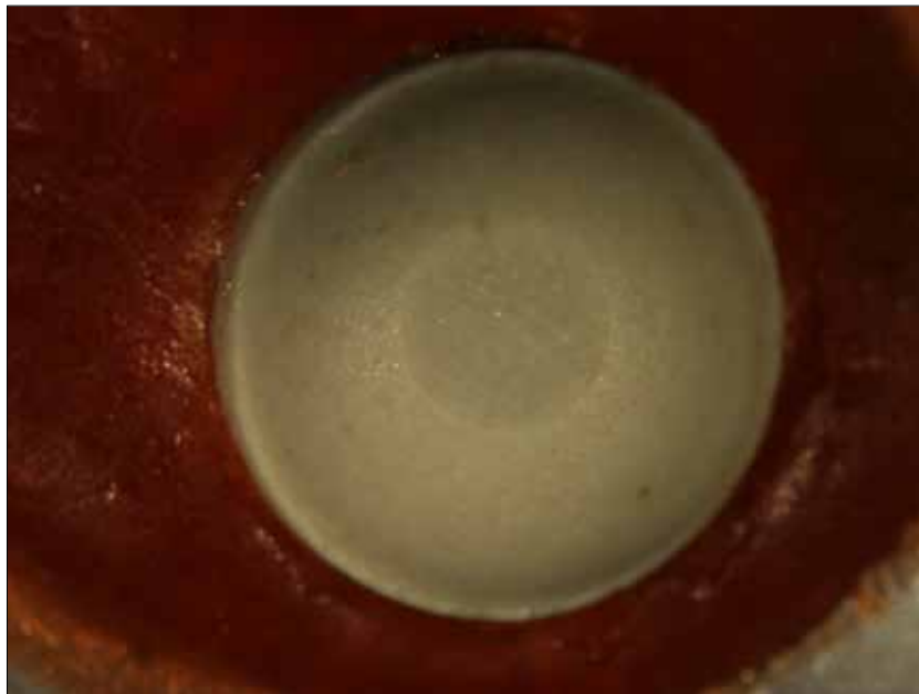
Fig. 8: Situation of the antagonist after the wear test in contact with Ceramco ® 3 (sample No. 6).
