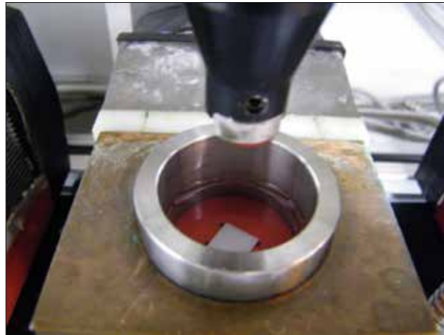
Fig. 1: Sample in test cell with antagonist/Steatite ball holder (top).
