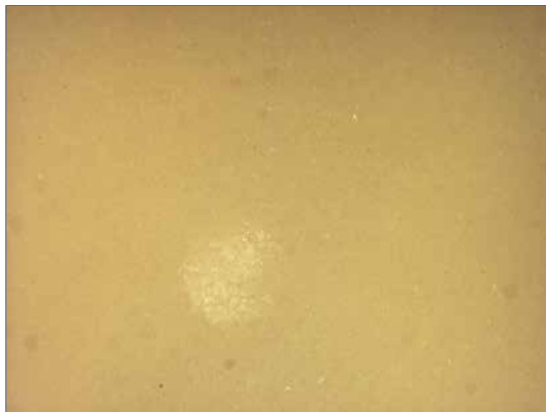
Fig. 6: Ceramco ® 3 after wear test (sample No. 4). The contact area is indicated by the bright spot.
