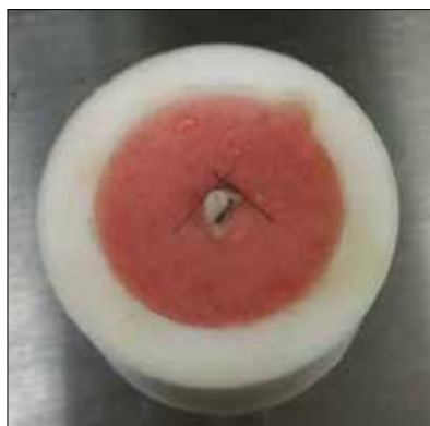
Fig. 2. Human premolar cusps embedded in acrylic resin (self-cure) in the lower sample holder.
