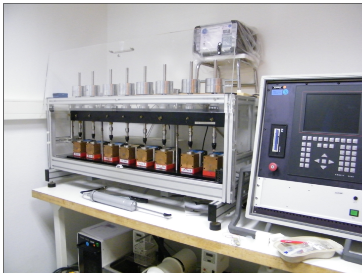
Fig. 2: Assembled test devices in the chewing simulator .
